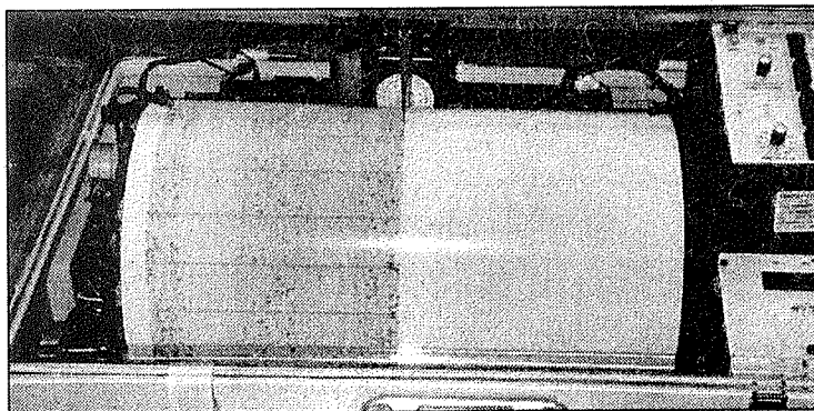
Seismograph at USGS records earthquake activity.
